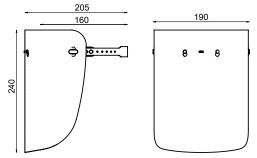
The shield is delivered disassembled for efficient handling and transport. The supporting part of the shield is made by plastic injection. Unique locks are designed for quick assembly and stable attachment of the visor to the supporting part with the possibility of easy replacement. Adjustable silicone headband and flexible carrying part ensure a comfortable fit for different head sizes.
